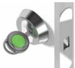
4. Insert the green finishing key of programming into the lock *once*. The key turns.
