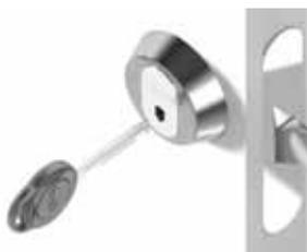
2. Insert the user key to be removed into the lock *once*. The key turns.
