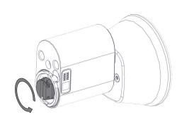
C. Remove the fixing screw. The tail plug can now be adjusted.
