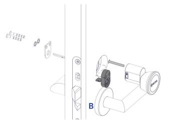
A. Remove the tail piece from the tail plug
