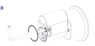
B. Loosen the tail plug fixing TORX10 screw by turning it carefully to the left.
