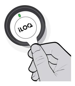
2. Turn the lock-reader knob to unlock the door.
