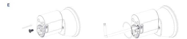
E. After adjustment, tighten the TORX10 screw again.
