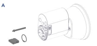
A. Remove the tail piece and the holding spring. Be careful when removing the spring.
