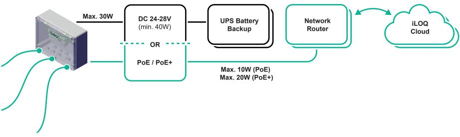
Figure 2. Bus power supply options and max. available bus power
