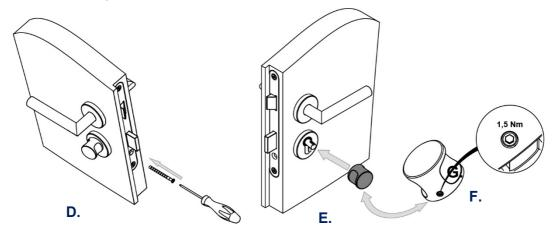
D. Fix cylinder into lock case by iLOQ fixing screw (A10.64, part of the delivery), use tightening torque 0.9...1.1 Nm. If necessary, cut the screw to the correct length (calculation screw length: L = backset + 10 mm).
