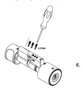
E. Insert the lock unit with extension piece back to the backbone of the cylinder housing. Fix the lock unit into the cylinder by 3 fixing screws. Tighten screws. Use tightening torque 0.55 ... 0.65 Nm.
