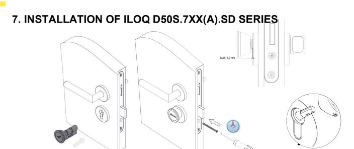
A. Ensure the cam is pointing downwards. Slide the lock cylinder through the lock case.
