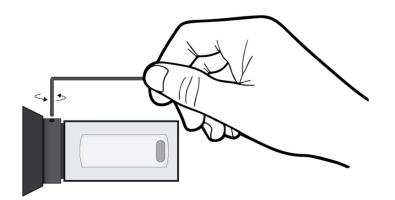
1. Loosen the knob screw by using the TORX 10 tool
