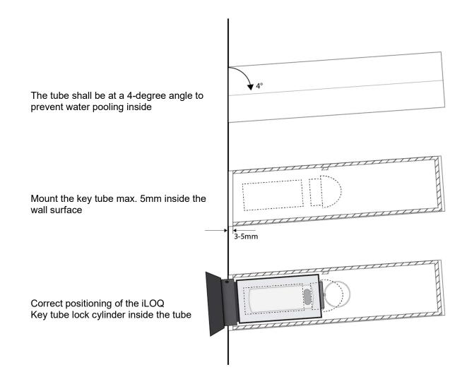
In case an existing key tube is mounted too deep inside the wall and the iLOQ Key tube cylinder cannot be placed in the key tube, it is possible to replace it with a version with a longer version. Please refer to the instructions on the next page and the documentation of the key tube manufacturer.
