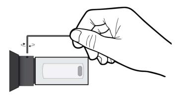
**4.** Tighten the screw by using the 1.5 Nm torque. Ensure that the head of the screw goes into the hole completely. A visible cap indicates that the screw is not in the right place
