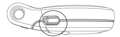
Nominal charging 5V, 100mA, time up to 3 hours depending on charger used for empty battery. Battery capacity 150mAh.
