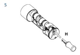
H. Insert the knob assembly key.
