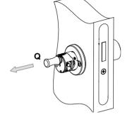
**Q** Remove knob assembly key.
