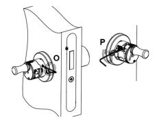
O. Mount with screw. Use tightening torque 0.15  $\dots$  0.2 Nm.
