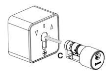
**C.** Fix the cylinder into a key switch according the key switch manufacturer's instructions.
