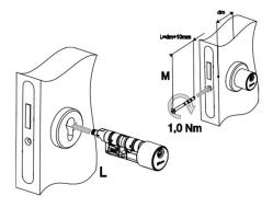
L. Slide lock cylinder through the lock case.
