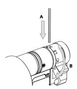
**A.** Adjust the cam position if necessary by pushing the locking pin for example with a TORX 6 tool from the iLOQ tool set.
