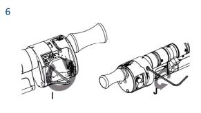
I. Remove screws both sides using TORX 6 tool.
