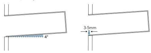
See the correct positioning of the F50S Key Tube Lock Cylinder inside the tube from the following image
