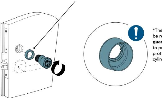
\*The security ring could be replaced by a **high guard escutcheon** to provide an extra protection to the cylinder and the knob.
