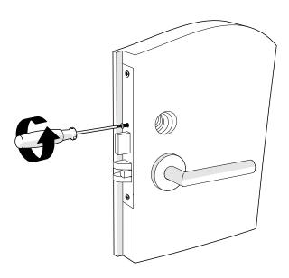
2. Thread the ILOQ cylinder with the security ring into the mortise lock.
