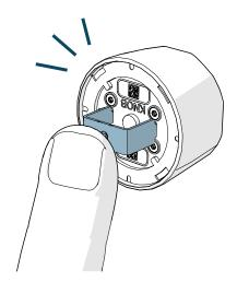
5. Slide the knob into the cylinder, push the knob until it stops. Remove the tool from the knob.
