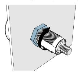
3. Install the latch, locking washer and latch fixing nut (3 Nm torque).
