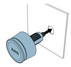
3. Install and tighten the security nut to a torque of 8 Nm.
