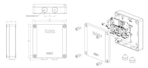
The iLOQ N501 Standalone Door Module is a device located in the vicinity of a door, and it controls devices installed on the door, such as a lock cylinder, an iLOQ NFC Reader, an electric lock, an electric strike plate, a magnet lock, and so on. The iLOQ N501 Door Module is equipped with a pre-installed 4G connection to the iLOQ Cloud. With the iLOQ N501 Door Module, the remote or otherwise hard-to-wire door environments can be easily connected to be a part of the iLOQ Online system.
